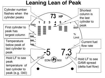
In the "lean of peak" method the columns will **invert** with the first to peak progressing down from the top of the display. The inverted column scale is  $5^{\circ}$  **per segment** below peak. As you continue to lean past peak the dot of the each successive cylinder will flash as it peaks. The peaks
