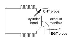
From the cockpit you can adjust the fuel/air ratio by a process called *leaning*. Retarding the mixture control changes the fuel/air ratio and hence the resulting Exhaust Gas Temperature (EGT).
