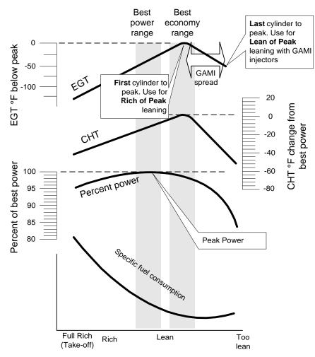
As the mixture is leaned, EGT rises to a peak temperature, and then drops as the mixture is further leaned. Peak *power* occurs at a mixture using more fuel than at peak EGT. Best *economy* occurs at peak EGT. Accurate leaning yields optimal engine temperatures. By being able to precisely adjust the mixture, your engine can produce either the best fuel economy or maximum power, whichever you choose.
