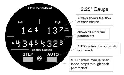
Two operating buttons control all functions of the FS-450M.
